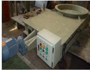
Motorized Slide Gate
