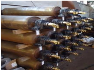
Discharge Roller Table – Transfer Roller
